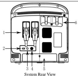
1. Probe 2.USB 3.Remote 4. Video Out 5.Battery Holder 6. Probe Holder
